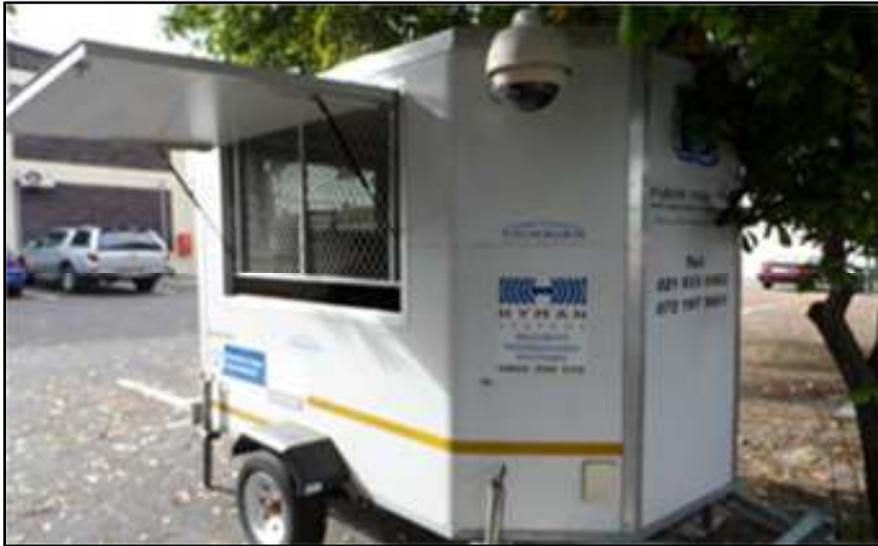
**Trailer equipped with cameras and an on-board DVR recording device offering mobile surveillance for instant deployment at “hot spot” areas.**
